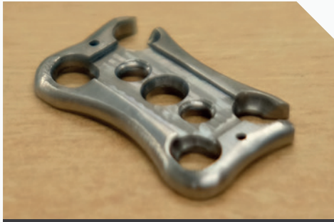
Implant plate programmed with ESPRIT and machined in a single operation on a 5-axis lathe.
