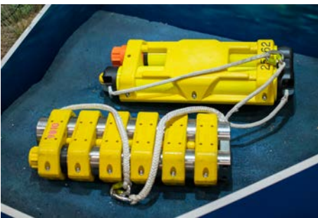
The final sensor. At the top is the plastic version for shallow water. At the bottom is the titanium version for deep ocean water.
