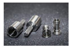
Modified handle and adapter programmed with ESPRIT and machined on a Tsugami BO326.
